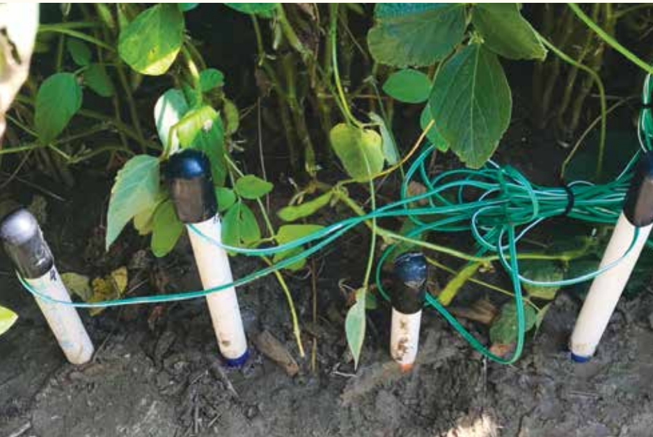
Soil moisture sensors that signal when to start and stop irrigation are installed in this soybean field at depths of 6, 12, 24 and 36 inches. Photo by Drew Gholson, Mississippi State University Extension
